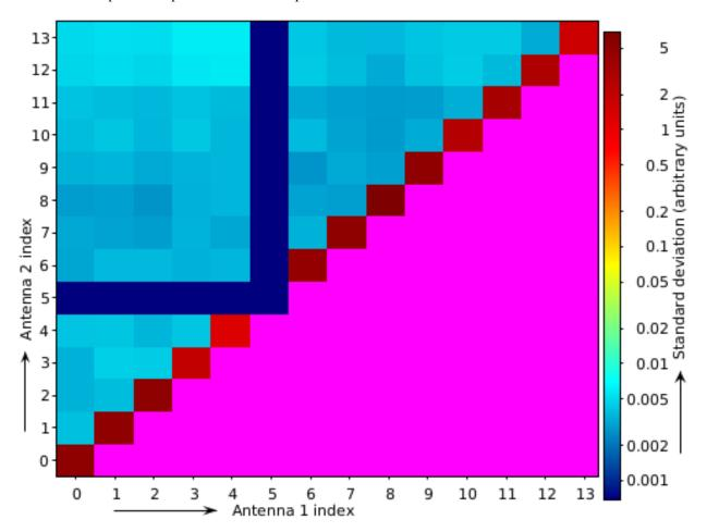
As can be seen from this image, antenna index 5 (WSRT RT5) is not working, and the autocorrelations show more power (as they should). Note that applot uses the quality statistics tables inside the measurement set. These are normally produced by tools like DPPP, cotter or aartfaac2ms; however, if a measurement set is not produced by one of those tools, it is necessary to create these tables manually. This can be done with the appuality collect <obs.ms> command.
