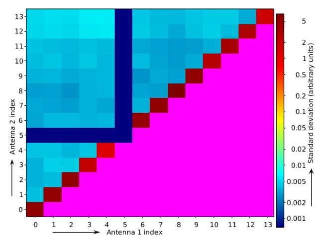
As can be seen from this image, antenna index 5 (WSRT RT5) is not working, and the autocorrelations show more power (as they should). Note that applot uses the quality statistics tables inside the measurement set. These are normally produced by tools like DPPP, cotter or aartfaac2ms; however, if a measurement set is not produced by one of those tools, it is necessary to create these tables manually. This can be done with the applainty collect <obs.ms> command.
